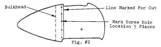
NOTE - You are now ready to apply Primary Fixturing which will require drilling holes in the side of the fairing. These holes will later be filled and will not be evident in the finished product.
