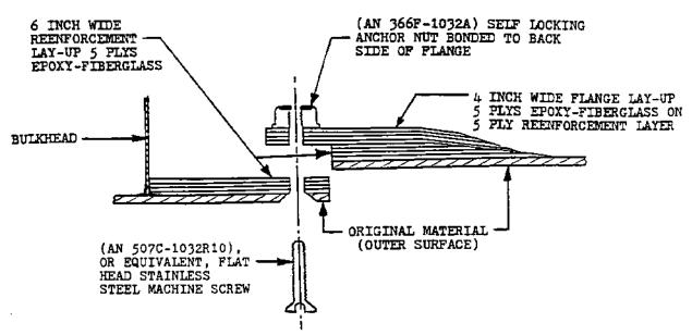
FIBERGLASS CLOTH - PPG 10 02. BI-DIRECTIONAL 18 THREADS PER INCH, OR EQUIVALENT LAMINATING/BONDING RESIN - FOLLOWING, OR EQUIVALENT, RESIN SYSTEM -
